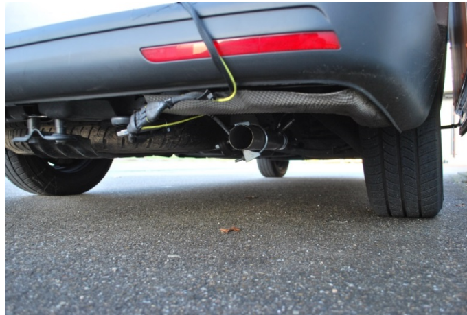
Figure 1: NO x sensor and thermocouple mounted in the vehicle's tailpipe.
