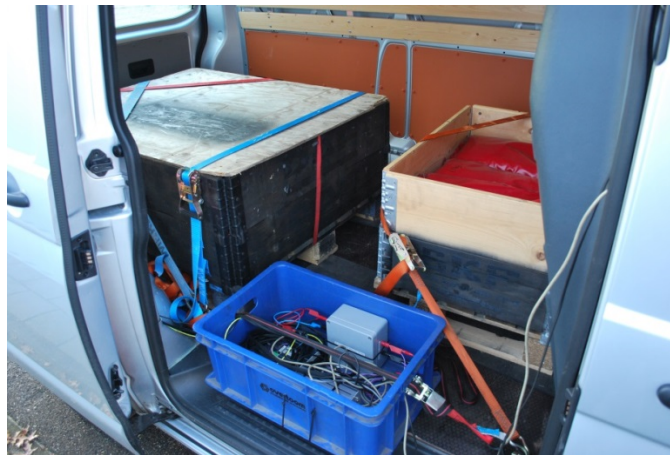
Figure 2: Load packages (black box) and data logger of the SEMS (blue cradle).
