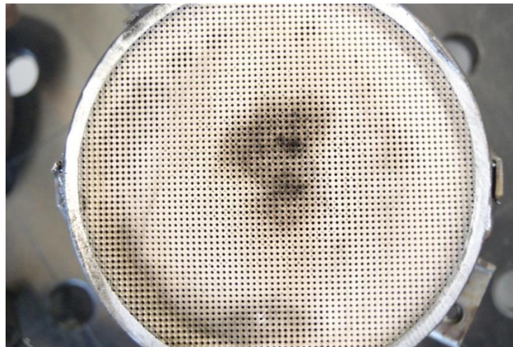
Figure 3: Backside of a cracked DPF of a Euro 5a diesel vehicle @ 160,200 km.
