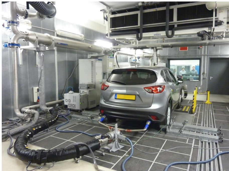
Figure 1: Emission test on a chassis dynamometer.
