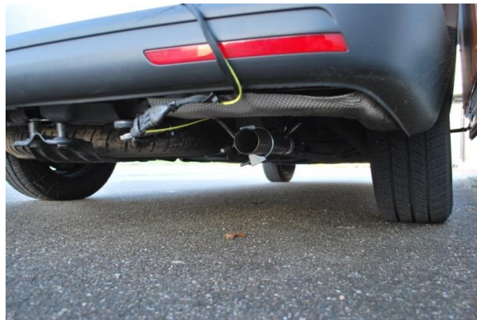
Figure 6: NO x sensor and thermocouple mounted in the vehicle's tailpipe.
