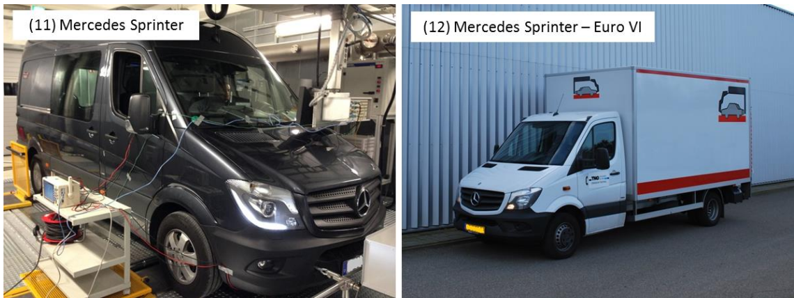
Figure 11: Pictures of the Euro 5 Mercedes Sprinter that was tested on the roller bench only as part of a European test programme exploring the correlation between NEDC and WLTP (vehicle 11 in Table 3 and Table 4), and of the Mercedes Sprinter that was equipped with an engine that was type approved under the Euro VI regulation for heavy duty vehicles (vehicle 12 in Table 3 and Table 4).
